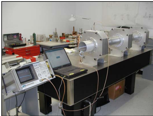
Figure 3: SRF injector cold model undergoing testing
