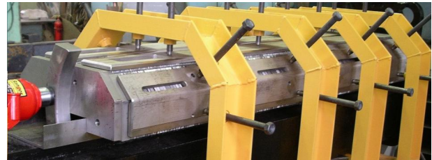
Figure 3. Dipole half yoke assembled before welding.
