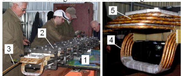
Figure 4. Dipole coil winding process.
