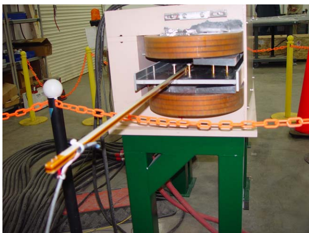
Figure 7. Measurement of modified septum by a flip coil.
