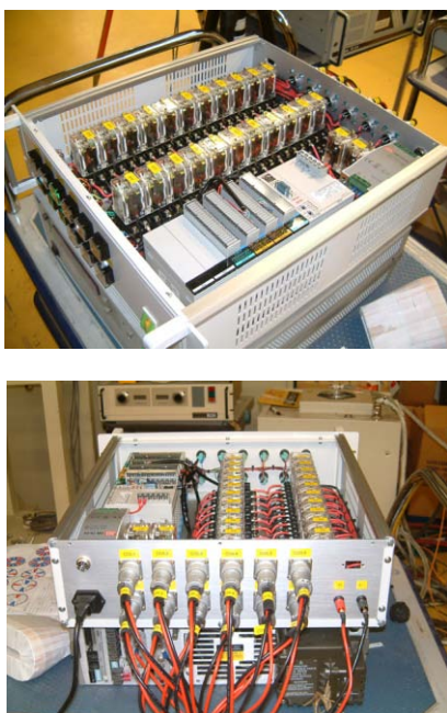
Figure 3: Instrument case of the power supply control system.
