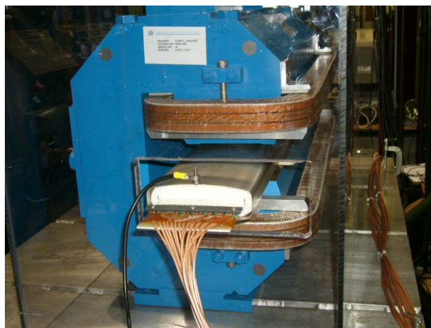
Figure 1: Circuit board probe array in C-magnet
