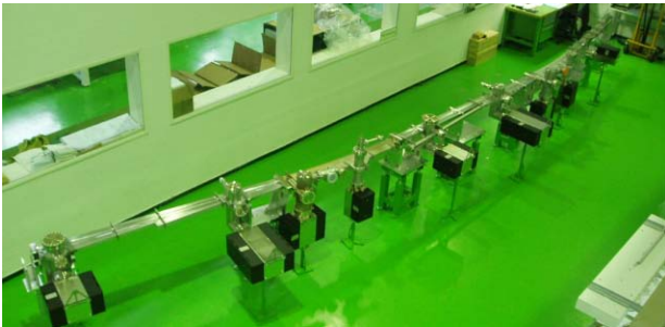
Figure 2: one complete cell assembled and ready for transport to the bakeout oven
