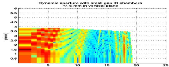
Figure 9: Dynamic aperture at long straight middle in the presence of multipole field errors and ID gap size of  $\pm 5$  mm, and 12 m in long straights and 5 m in standard straights.
