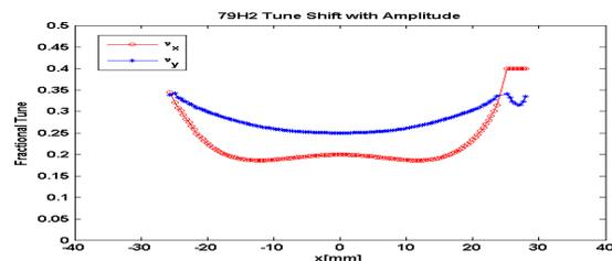
Figure 3: Tune shift vs. horizontal amplitude.
