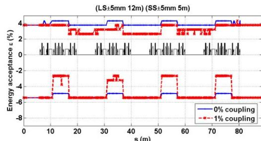
Figure 11: Energy aperture in one superperiod.
