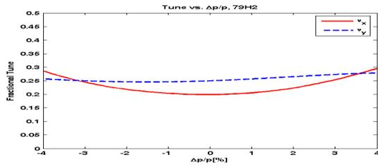
Figure 4: Tune shift vs. energy deviation.
