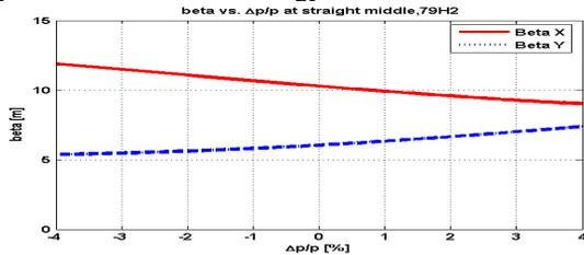
Figure 5:  $\beta_{x,y}$  at long straight middle vs. energy deviation.
