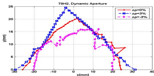
Figure 6: Dynamic aperture tracking for on-energy and off-energy particles at long straight center.
