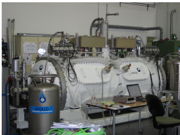
Figure 4: SOLEIL module at the final test at ACCEL. The module is cooled down to 4 K and the cavity frequency is checked and the right damping of the HOM couplers is measured.
