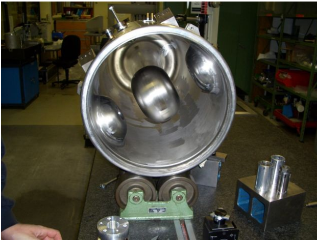
Figure 8: Look into inside of medium beta 88 MHz quarter wave resonator for GANIL. The cavity is in the dimensional control workshop and already completed with helium vessel at this stage. Only one more weld to close the cavity at the bottom is missing.
