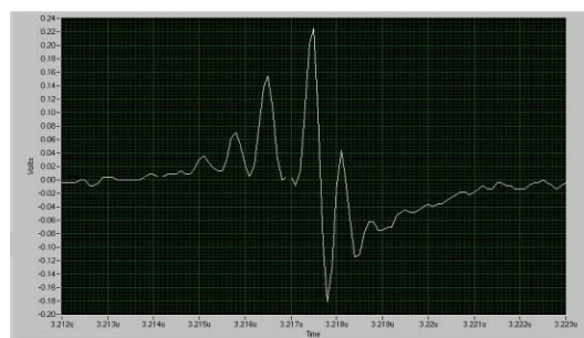
Figure 4: Difference signal from a button BPM showing an instability with a frequency of 2 GHz. The horizontal scale spans 11 ns. (Run-8 non-operational test ramp with d .)
