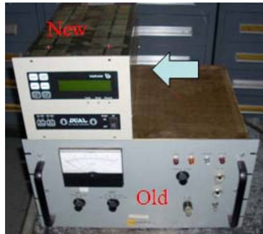
Figure 3: Comparison between a new ion pump power supply for 500 L/s ion pumps and our old one.
