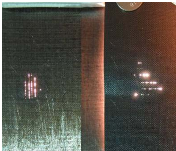
Figure 4. SNS secondary carbon/carbon foil after a 3-month run cycle. The foil halves (left, \text{H}^0 ; right, \text{H}^+ ) have been pieced together for this image.
