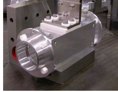
Figure 3: A photograph of the small drifttube
