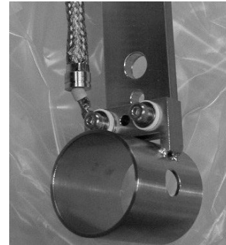
Figure 4: Post acceleration tube and aperture plate
