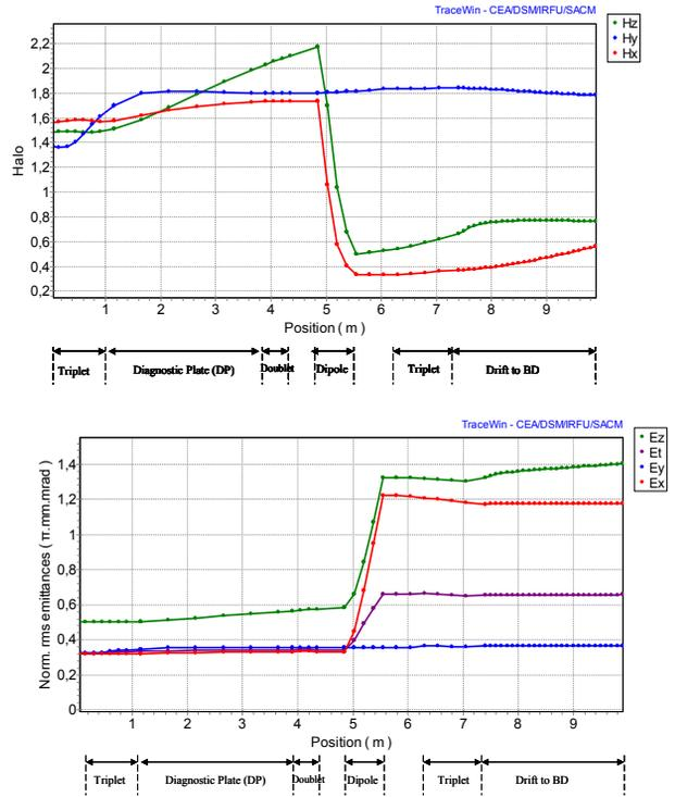
Figure 4: Halo (up) and normalized rms emittance (bottom) in the HEBT. X and y are the transverse coordinates whereas z is the longitudinal one.
