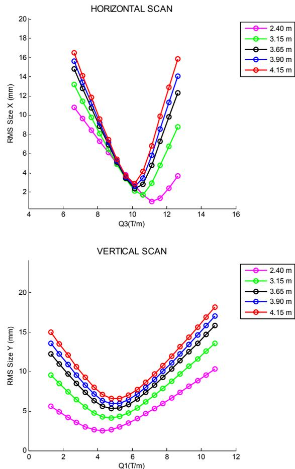
Figure 1: Quadrupole scan for transverse emittance measurement. RMS beam size as a function of the quadrupole gradients (first quadrupole for the horizontal direction and third for the vertical one). The different curves show the rms sizes at different locations from the input of the HEBT.
