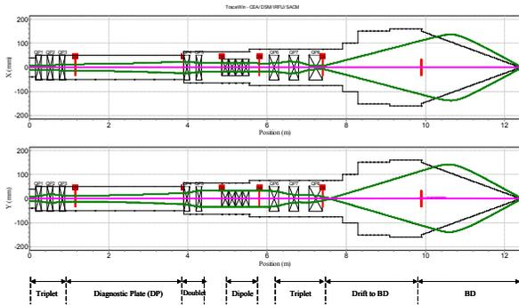
Figure 2: 3 RMS envelope for HEBT line.
