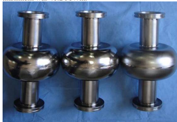
Figure 1: Cavities (Left two: China Ningxia Large Grain Niobium; Right: China Ningxia fine grain niobium) with the IHEP low loss shape fabricated at IHEP.
