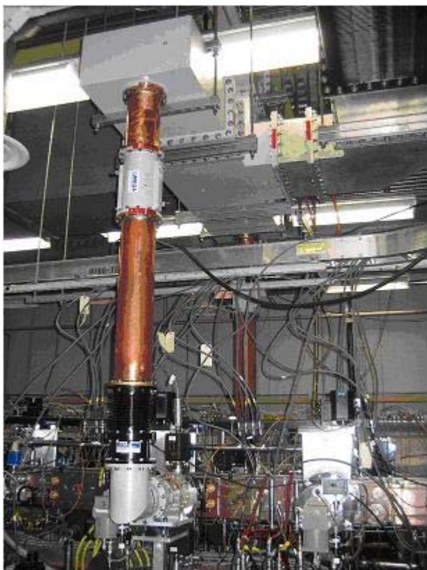
Figure 4 – Upgraded coupling system of the RFQ.
