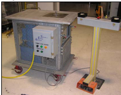
Figure 1: AES Designed & Built Branch Pulling Machine
