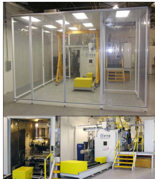
Figure 3: EB Welding System at AES
