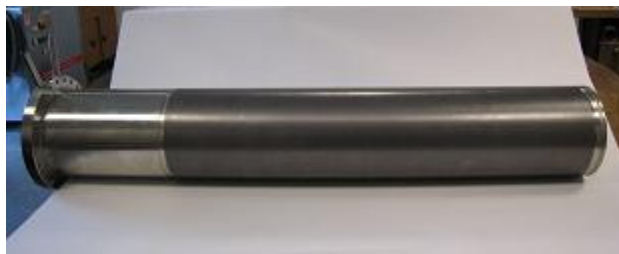
Figure 3: The MS-ECRIS plasma chamber.
