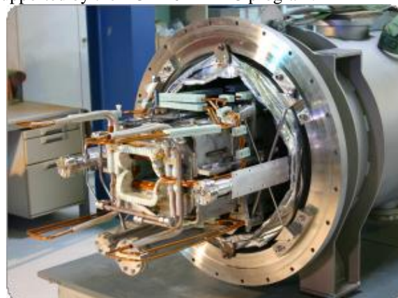
Figure 2: Straight SIS100 full length model dipole magnet manufactured at BNG (Würzburg).
