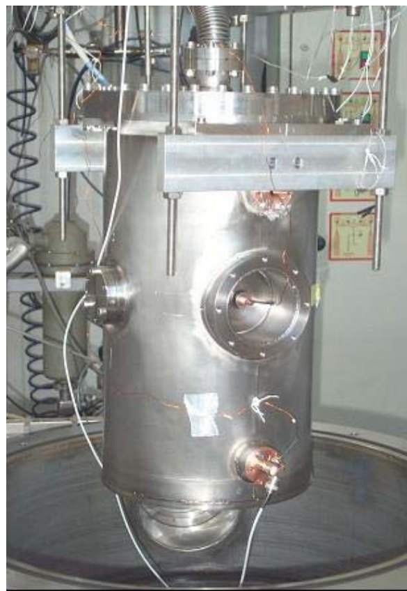
Figure 1. The \beta_0=0.31 , 352 MHz HWR mounted in the test cryostat.
