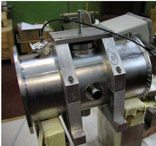
Figure 3. Final frequency adjustment: tuning cup position adjustment before final welding.
