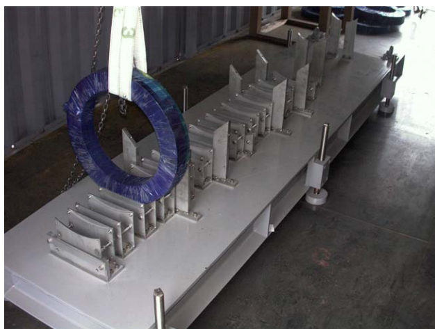
Figure 9: Fabricated Supporting Structure
