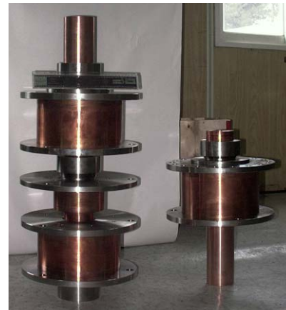
Figure 7 : Pre-assembled RF cavity
