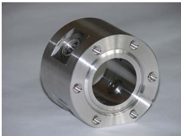
Figure 1: The vacuum body of the button BPM.
