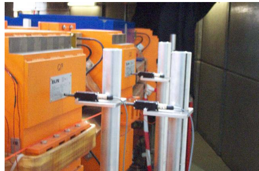
Figure 2: Installation of sensors before quadrupole magnets.
