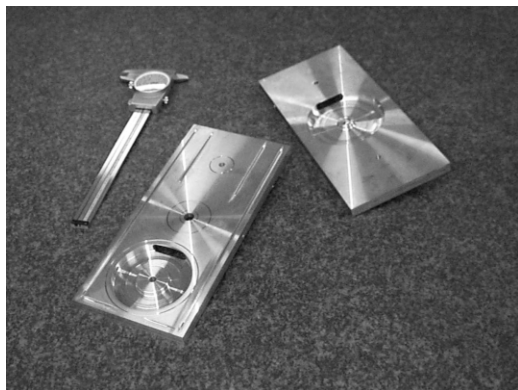
Figure 2: Half-cell-plates showing a coupling half cell (left) and an accelerating half cell (right). Note the coupling slot.
