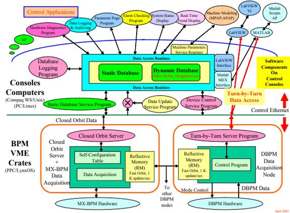
Figure 3: Software environment for DBPM data access.
