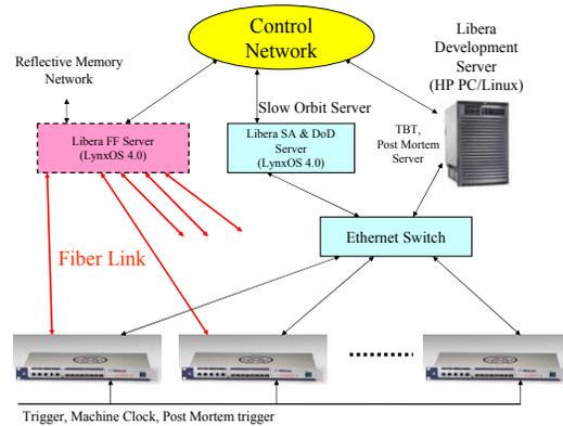
Figure 4: Block diagram of Libera data access.
