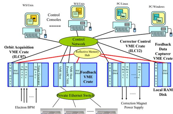
Figure 1: Software environment for BPM data access.
