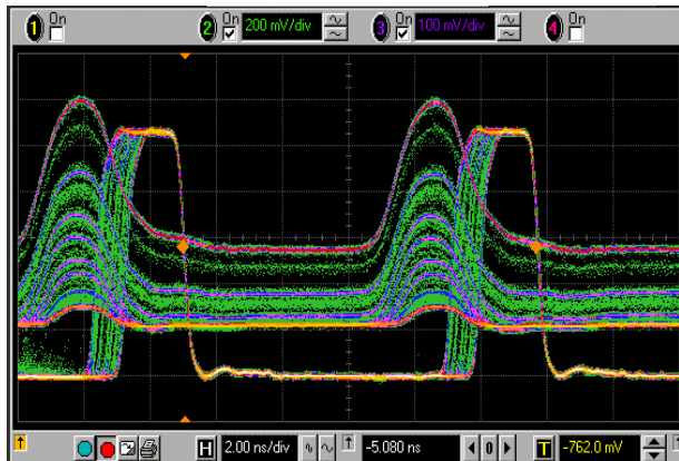
Figure 2: Output response of the LHC beam position monitor fibre-optic link.
