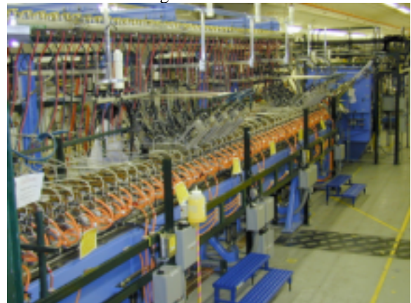
Figure 1. The 11-m, 52-magnet FODO lattice includes nine WS/HS stations that measure the beam's transverse projected distributions.
