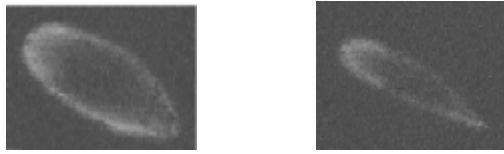
FIGURE 2. Images of ^{40}\text{Ar}^{+7} beam with solenoid focusing. On the left, helium used as a support gas in the source. Shutting off the helium gas supply results in the image on the right. Peak of charge distribution is ^{40}\text{Ar}^{+9} .
