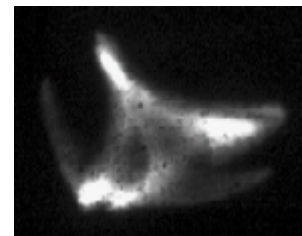
FIGURE 4. Image of ^{16}\text{O}^{+3} beam with electrostatic quadrupole triplet focusing under the SC-ECR. The distance between bright spots is 3 cm.
