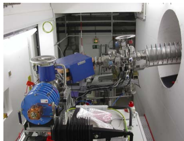
Fig. 3: New ion source platform: The 150 kV new platform with a 14.5 GHz Supernanogan ECR ion source is close to completion
