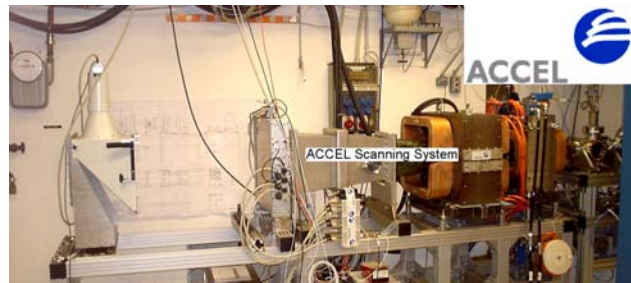
Fig. 6: The ACCEL nozzle and scanning test equipment installed at ISL
