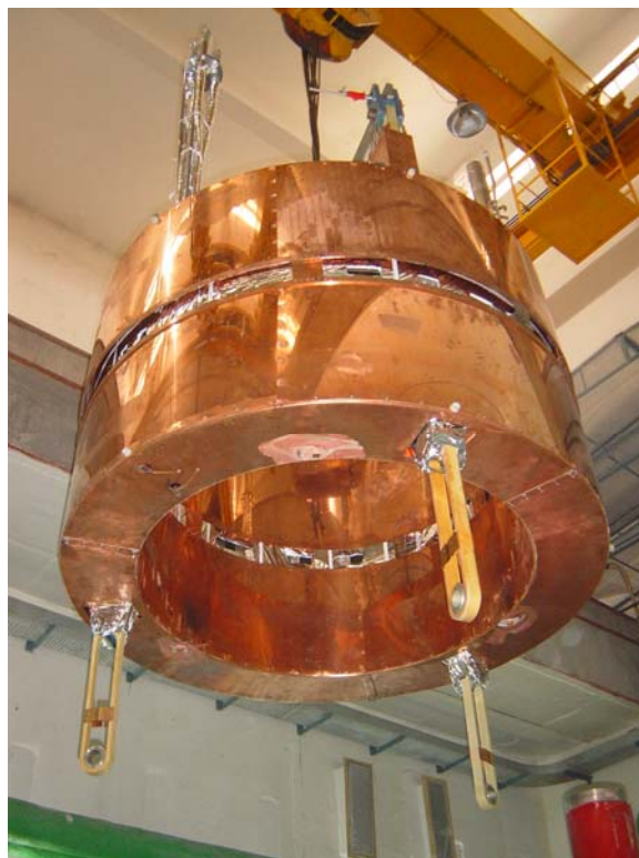
Fig 4: Cryostat bobbin with multilayer insulation and LN-2 cooled radiation shield.
