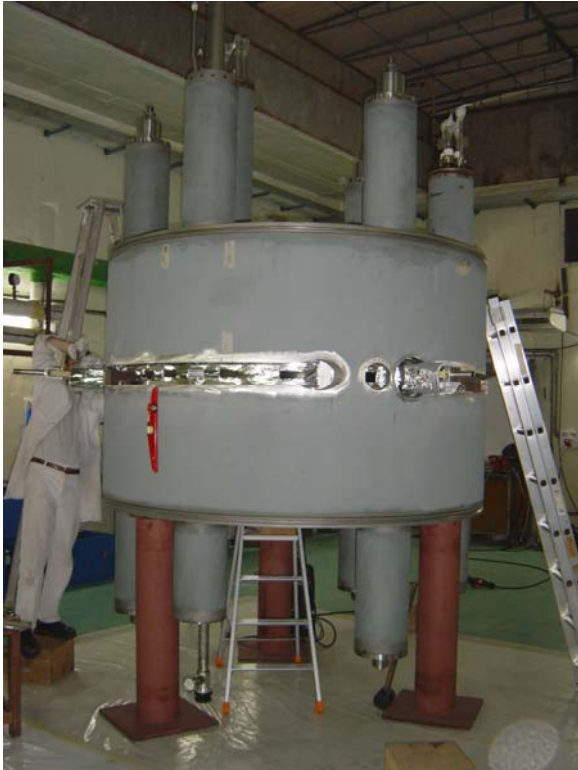
Figure 5: Final assembled cryostat without median plane inserts.
