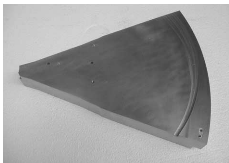
Figure 1: The removable pole tip with the evolved groove
