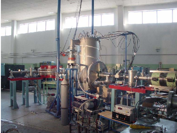
Fig. 6 Layout of proton beam accelerating structure
