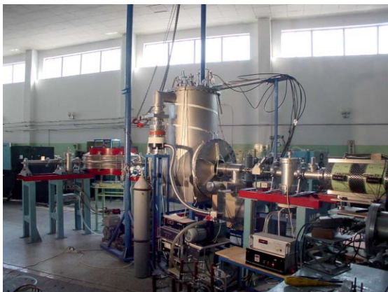
Fig. 12 The beam test of the Nb-Cu sputtered QWR
