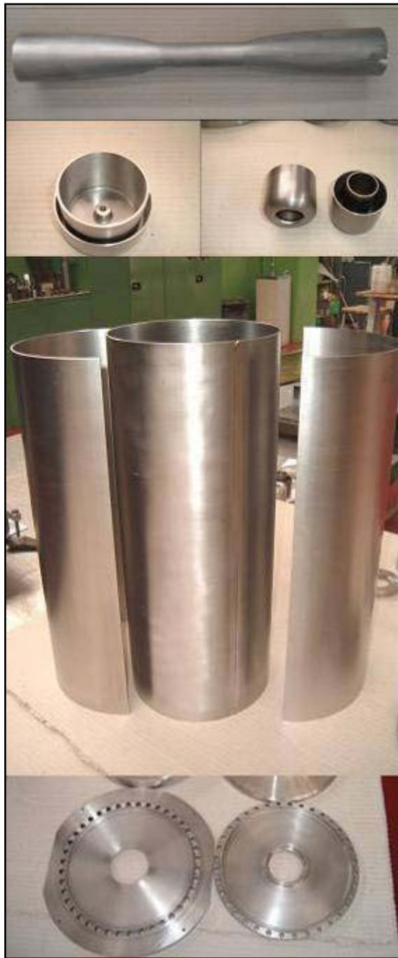
Figure 4: Parts of the low- \beta 352 MHz HWR under construction. From top: inner conductor, tuning cup, beam ports, outer conductor and outer vessel, shorting plates.
