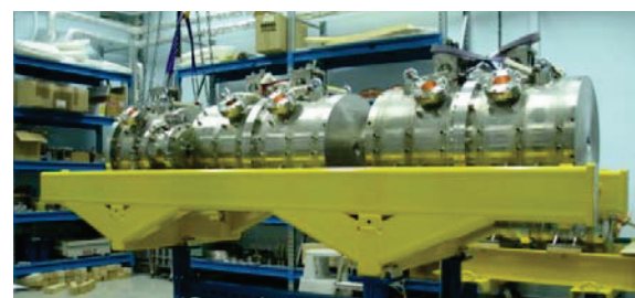
Figure 5: CCDTL module 2 during tests at Novosibirsk.
