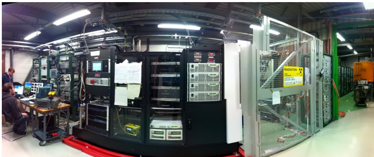
Figure 1: A photograph of the Xbox-1 test stand. The control and low-level rf systems are to the left, the modulator is in the middle and the high-power rf network is to the right. The test accelerating structure is located in the former CTF2 accelerator bunker located in the floor below.
