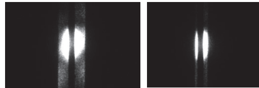
Figure 9: Target images using 0.5 mm target aperture and 2 mm (left), and 1 mm mask aperture (right).
