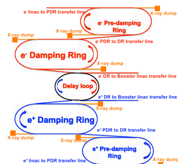
Figure 1: A schematic view of the DRs' complex, with blue DRs for positrons and red for electrons. A single delay and recombination loop (black) is used for both species.
