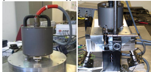
Figure 1: Two demonstration benches: left: single d.o.f. system (membrane), right: two d.o.f. system (tripod) with 100 kg dummy magnet mass.
