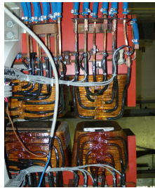
Figure 6: Coils connections in the DAFNE wiggler. From the right to the left the terminal and the central coils.
