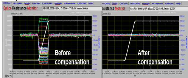
Figure 1: Busbar signals before and after compensation
