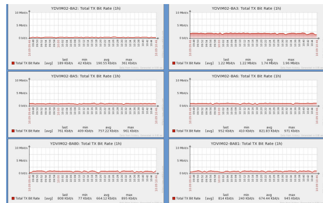
Figure 1: Transmit bit rates of several surveillance cameras of the SPS. Any anomalies can be spotted with a glimpse.
