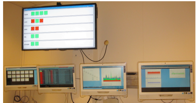
Figure 2: Screens showing various views of the monitoring system at the premises of the maintenance team: The large screen displays the overall system status and the small screens a collection of detailed graphs. The different views have been made to rotate to display as much information as possible.
