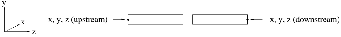
Figure 5.1: COMPASS coordinate system and illustration of the target centre coordinates given in Table 5.2. The origin of the COMPASS coordinate system is in the middle of the downstream target cell. The x -axis is the horizontal axis pointing towards the Jura, the y -axis points to the ceiling and the z -axis points downstream along the beam.
