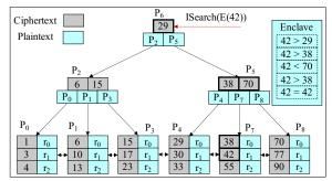
Figure 1: B<sup>+</sup>-tree with encrypted keys. Node ids  $(p_0-p_8)$  and record ids  $(r_0-r_2)$  are plaintext.
