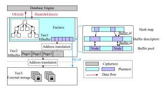
Figure 2: Three-tier architecture of Enclage Index.
