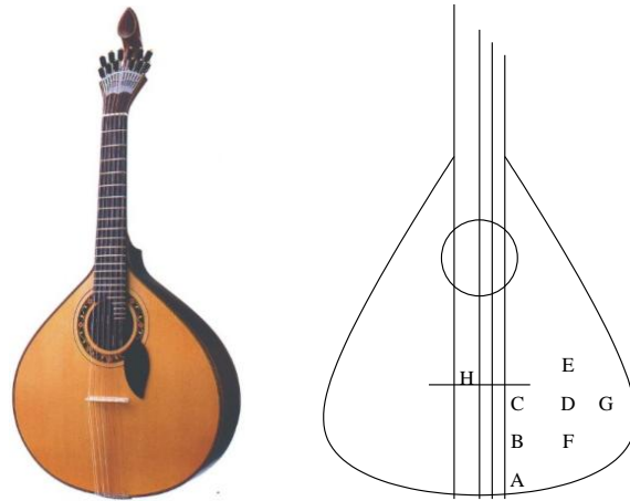
Figure 4: Picture of a Portuguese guitar and points hit during the experiment
