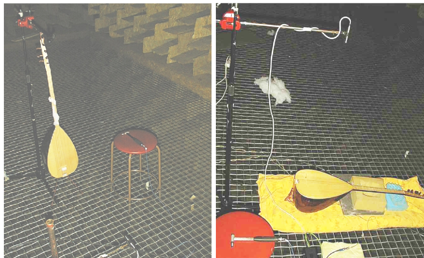
Figure 5: Two setups for measurements of the saz in anechoic chamber
