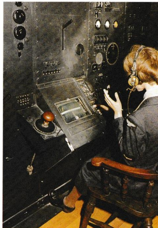
9 The 'girl on the tube' responsible for updating plots and watching for new echoes. Her left hand should be operating the goniometer, whose wooden handle is clearly visible. (courtesy the RAF Museum, Hendon)
