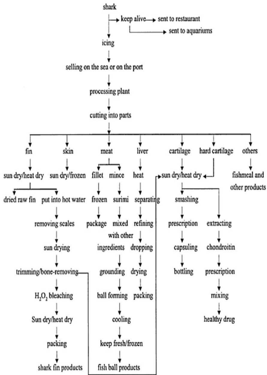
Figure 13: General shark processing flowchart (shark landed with fins attached)
