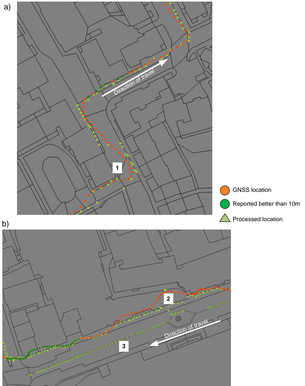
Figure 20: User moving along pavement, with original and processed position tracks displayed (a) and the road centreline snap point (b)
