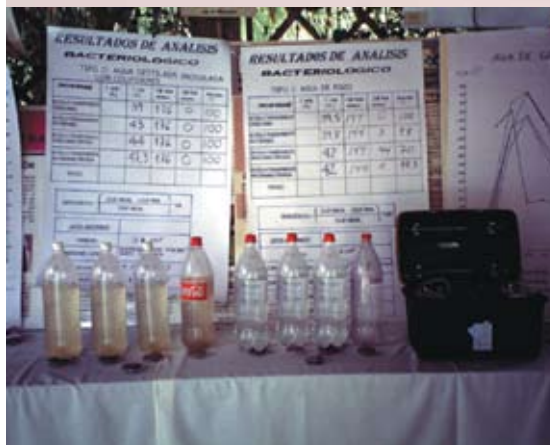
Water quality analysis using a DelAgua field test kit during the workshop to demonstrate SODIS efficiency.
