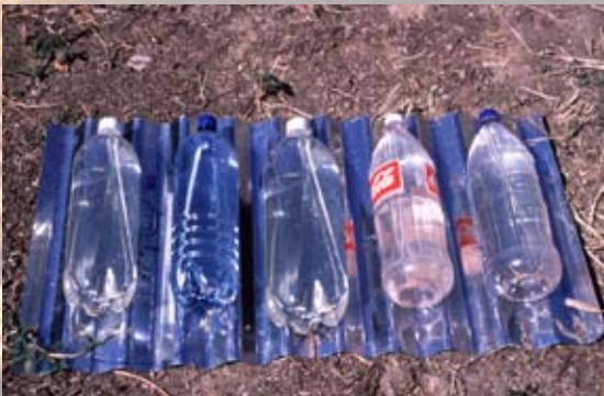
CGI-sheets reflect sunlight and therewith are an ideal bottle support for SODIS
