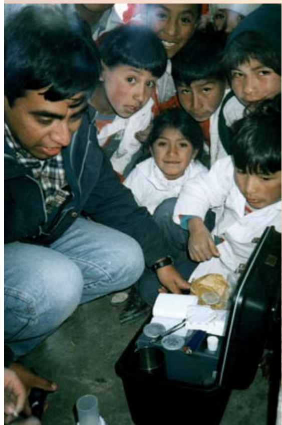
Using the DelAgua field test kit to examine the water quality
