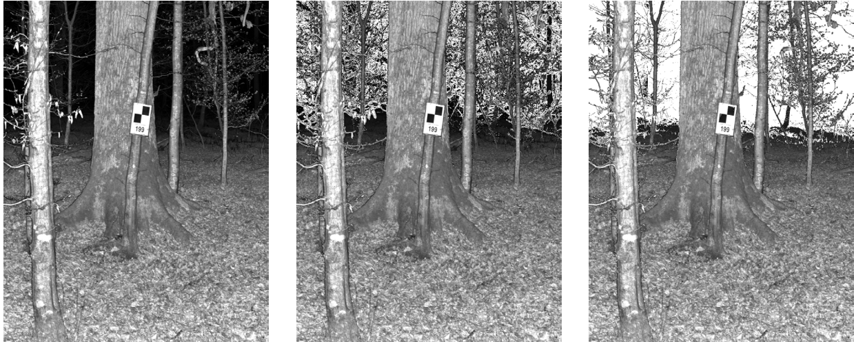
Figure 3a: Intensity Image of a scan; b: point cloud without isolated points, filter by a value of 2 metres; c: point cloud b filtered by points of an intensity less then 500 and more then 20,000.
