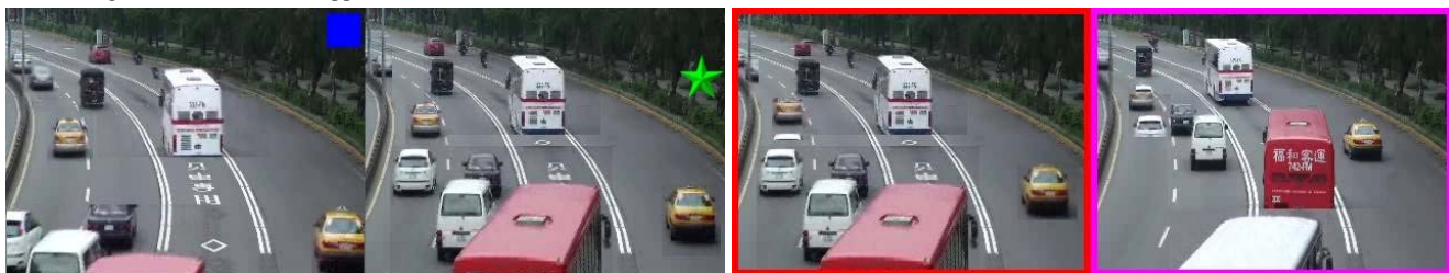
(a). Two consecutive compact frames with n=60 . The left and the right are generated by the source frames marked by a blue and green rectangle, respectively, in (c). (b). Two consecutive compact frames with n=120 . The left and the right are generated by the source frames in a red and purple rectangle, respectively, in (c).
